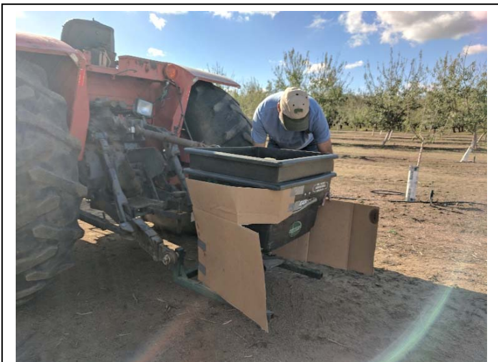
Figure 2: Modified ant-bait spreader used for seeding.
